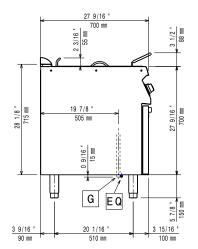
EQ = Equipotential screwG = Gas connection
